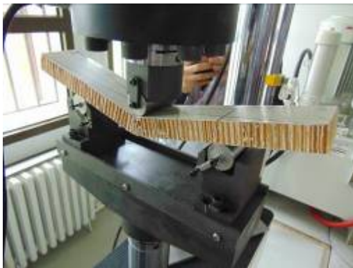
Figure 17. Loaded beam before top plate failure
