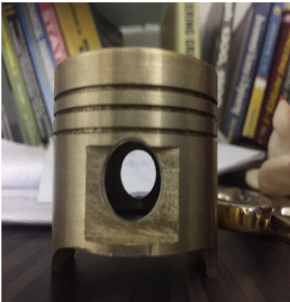
Figure 3. Piston made of composite material in vacuum stir casting.
