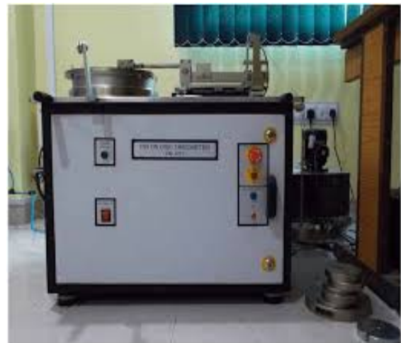
Figure 5. experimental setup of Pin on Disc
