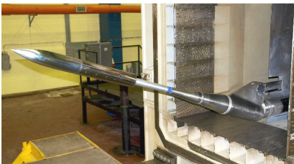
Figure 2. The 115.8 mm dia. AGARD-B model with 0.53% blockage in the T-38 wind-tunnel of VTI
