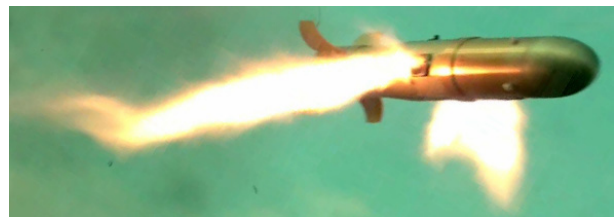
Figure 1. Missile with thrust vector control by tabs
