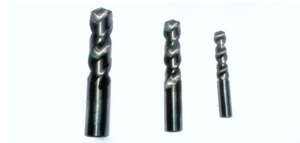
Figure 3. Drill bits of different diameters used for experimentation
