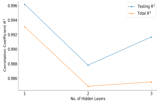
Figure 7. Comparison of R^2 values for different hidden layers for thrust force modelling
