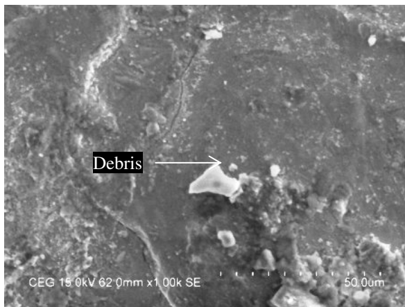
(b) Current = 10 A, Pulse-on-time = 150 \mu s, Pressure = 2.0 kPa (for LM13 aluminum alloy, I = 6 A)
