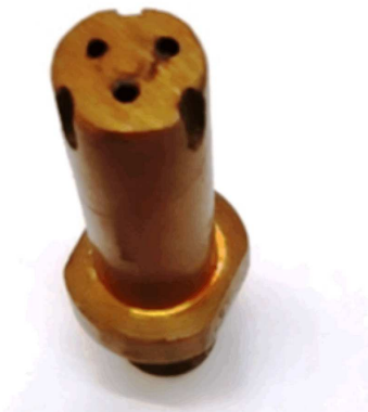
Figure 2. Drilled copper electrode with slots
