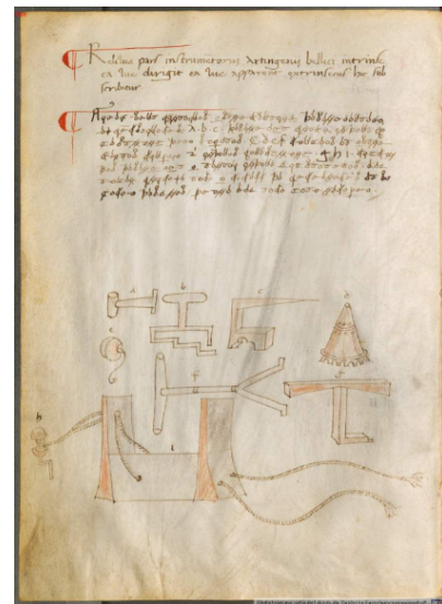
Figure 5. Parts of a lathe operated with a crank [22].
