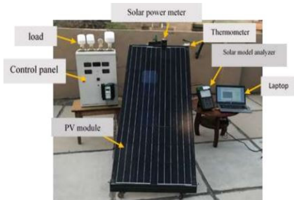
Figure 3. Experimental setup system with measuring device
