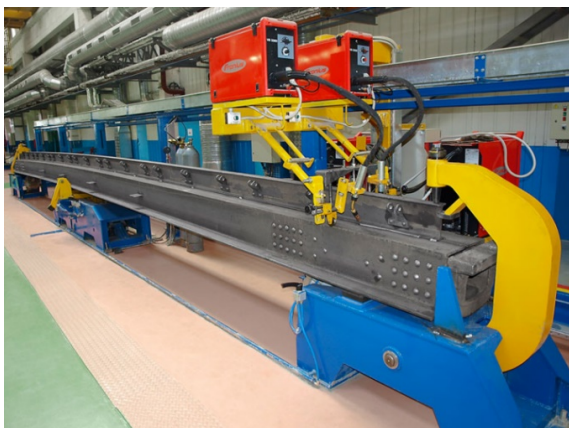
Figure 6. Robotic complex for manufacturing of the centre sill
