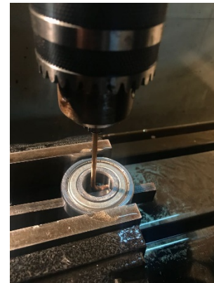
Figure 2. Inner race fault simulation method
