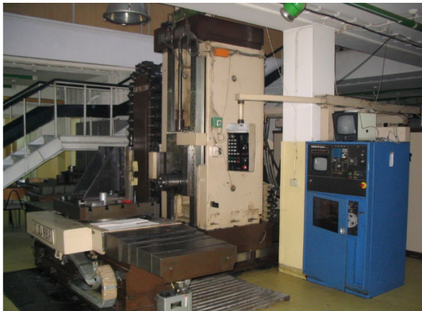
a) Original machine LOLA HBG 80 OC with Bosch control system
