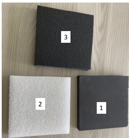
Figure 2. Foams used for this study, 1) XPE 30, 2) PE 25 and 3) PE30
