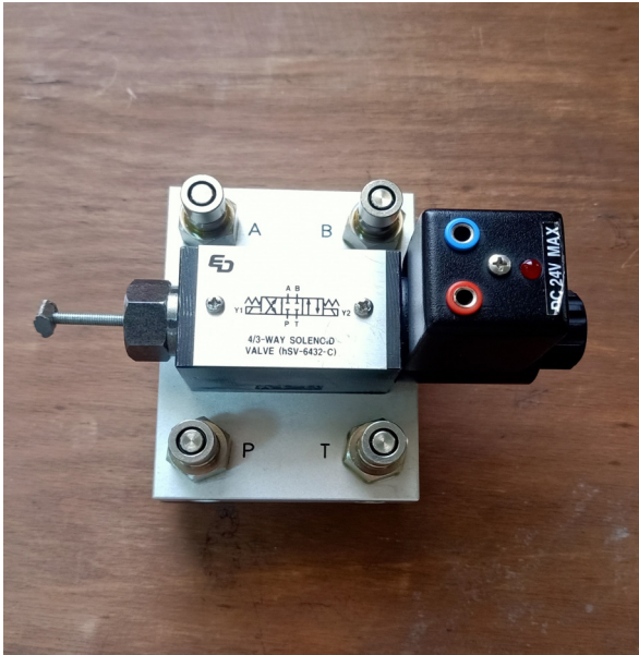
Figure 8 Modifications applied to the solenoid valve to be able to connect the LVDT.
