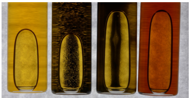
Fig. 5. The test-ready lubricant mixtures 4 days after the ultrasonic agitation. From left to right: 1. reference lubricant (Castrol EDGE 0W-30); 2. multiwalled carbon nanotube doped reference oil; 3. Graphene sheets doped reference oil; 4. C60 fullerene doped reference oil. The sediment is visible in the MWCNT doped and the graphene doped engine lubricating oil.
