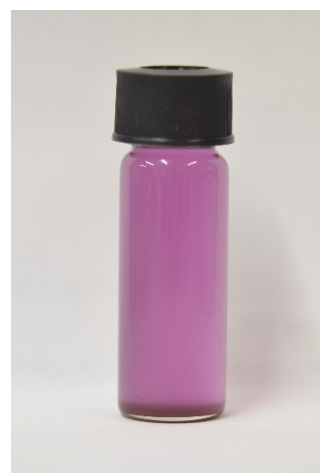
Fig. 3. C60 fullerene doped colorless base oil turned purple. The purple color is that the individual fullerene molecules absorb green light.
