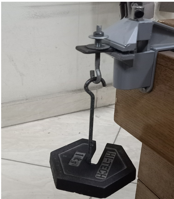
Figure 9. Experimental setup to measure the spring stiffness.
