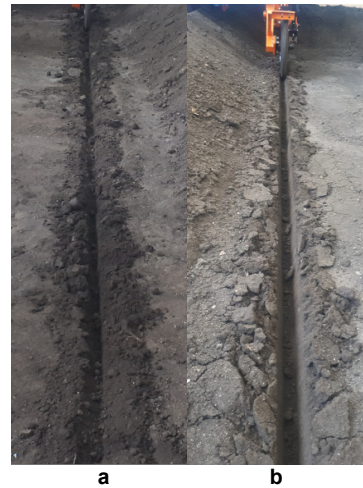
Figure 15. A furrow left after the passage of the sowing section: a - the sowing section with the installed slotting disk; b - the sowing section without the installed slotting disk
