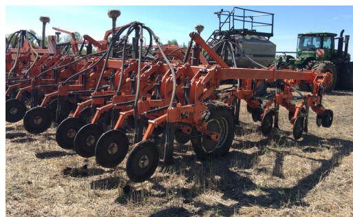
Figure 19. PK-12.7 sowing complex equipped with combined sowing sections
