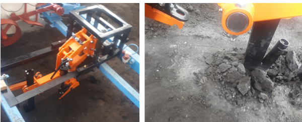
Figure 9. Determining the tractive resistance of the anchor colter of the sowing section
