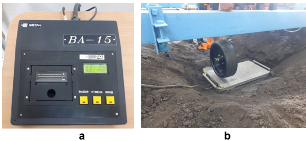
Figure 8. Static determination of the reaction acting on the balancing wheel using the VA-15 scales (a - remote control panel of the scales; b - scales platform)
