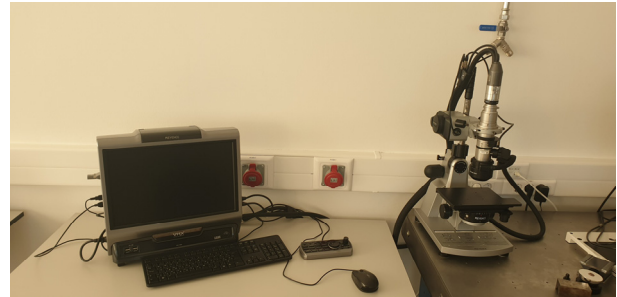
Figure 4. Keyence VHX-1000 digital microscope, which was used for measuring the wear scar dimensions on the testing specimens after the tribometer measurements (picture of the authors)
