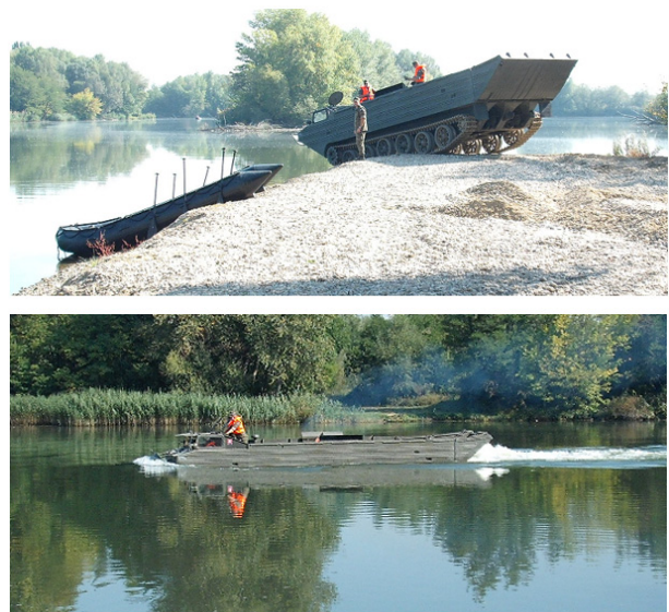
Figure 1. PTSZ-M military vehicle in land operations (top) and in water operation (bottom) condition (pictures of the authors)
