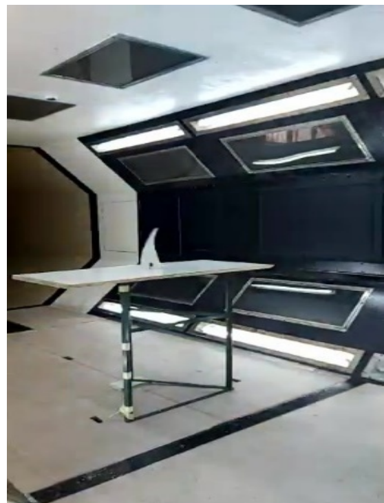
Figure 16. Wind tunnel flutter test
