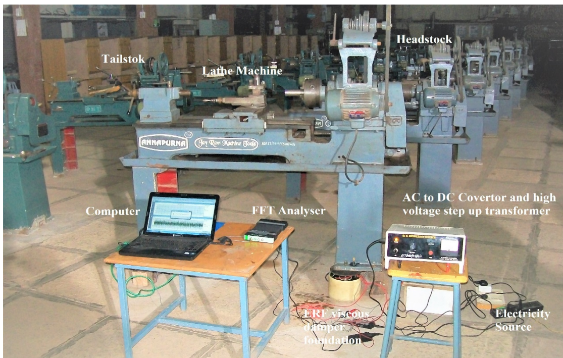
Figure 8 Experimental setup to obtain the response of the ERFMM used to mount a lathe machine (quarter machine model)
