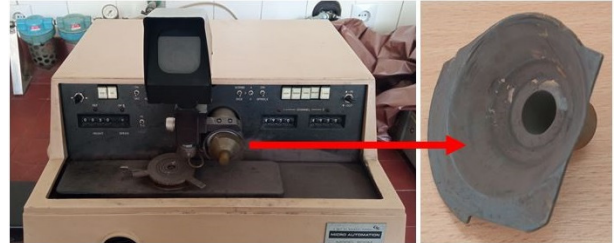
Figure 2. Micro Automation device for cutting silicon wafers (left) with a fractured protective cover (right)
