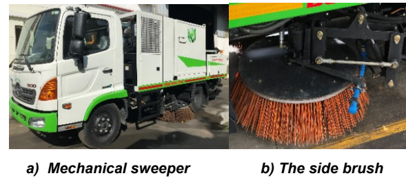
Figure 1. The mechanical sweeper and the side brush [23]
