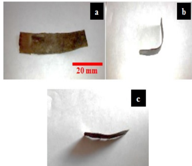
Figure 4. Photograph showing C1 alloy prior to bending, after bending, and shape recovery post-heat treatment.
