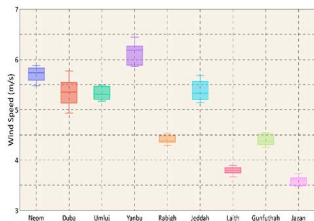
Figure 3. The yearly average wind speed (m/s) for the nine selected sites at 50 m
