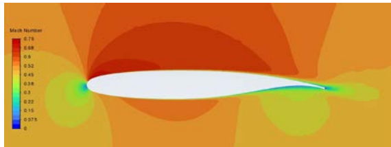
Figure 11. Mach number contour around NASA sc (2) 0712 at AOA 0° - 3D case
