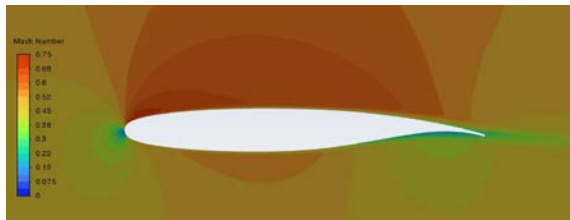
Figure 10. Mach number contour around NASA sc (2) 0712 at AOA 0° - 2D case
