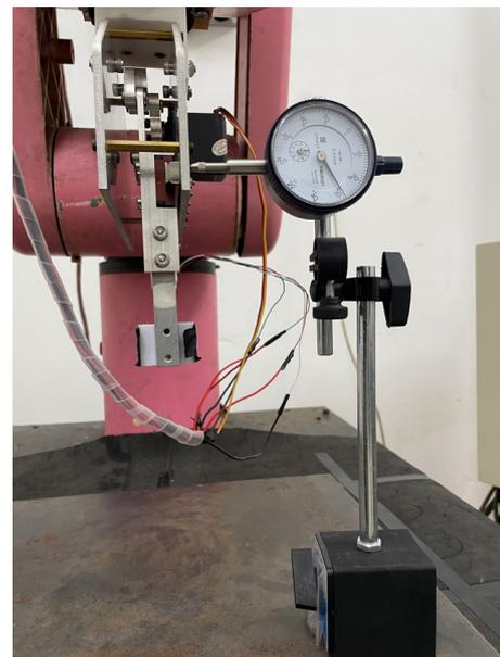
Figure 17. Experimental result of the measured error in Y axis.
