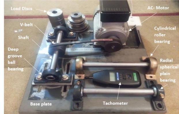
Figure 1. Experimental Rig.
