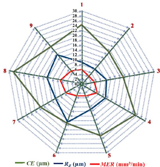
Figure 5. Variation in circularity error; mean surface irregularity depth; and machining erosion rate with machining combinations.
