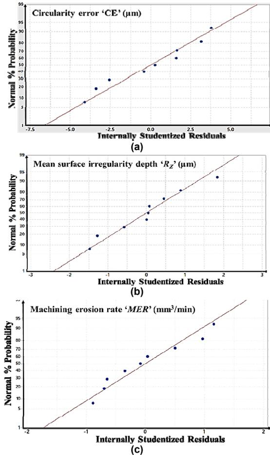
Figure 4. Normal probability graphs of selected responses: (a) circularity error; (b) mean surface irregularity depth; and (c) machining erosion rate.
