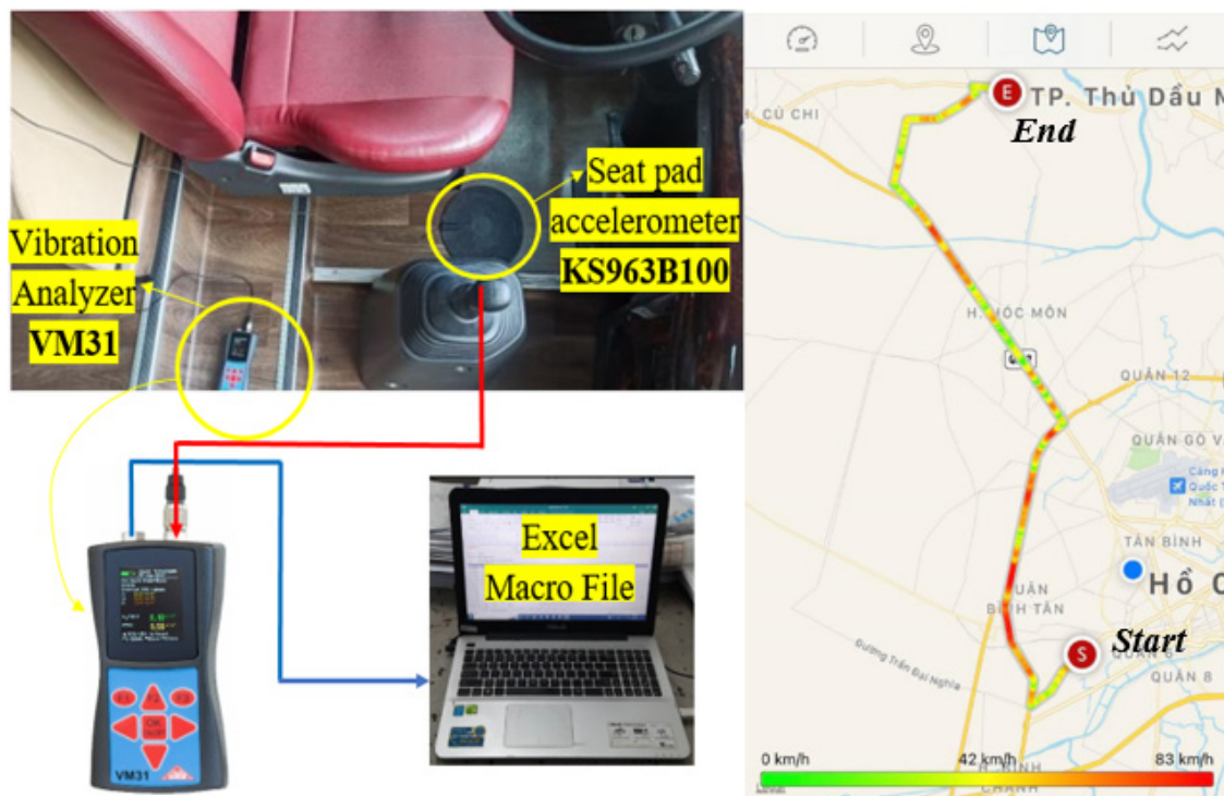
Figure 1. Experimental setup for collecting vehicle's floor excitation data
