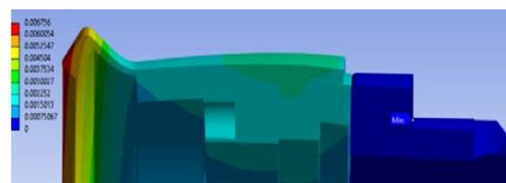
Figure 30. Deformations for a process fluid temperature of 40°C (scale of 1:620)
