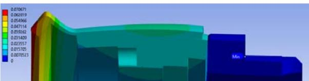
Figure 33. Deformations for a process fluid temperature of 200°C (scale of 1:63)
