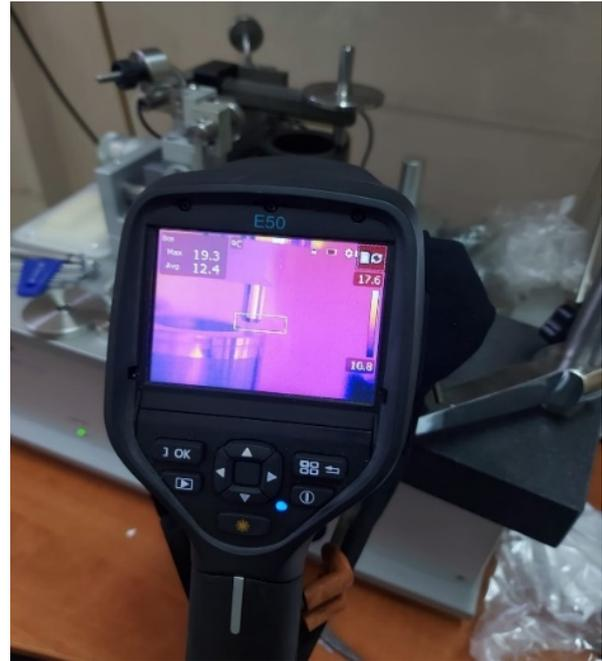
Figure 10. FLIR-50 measurement of temperature
