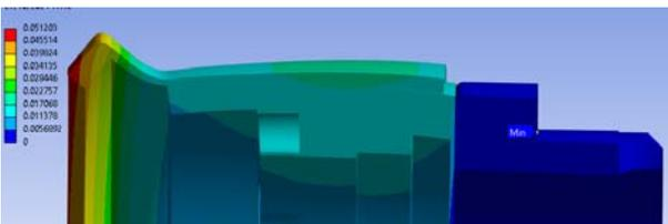
Figure 32. Deformations for a process fluid temperature of 150°C (scale of 1:87)
