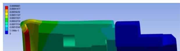
Figure 29. Deformations for a process fluid temperature of 22°C (scale of 1:390)
