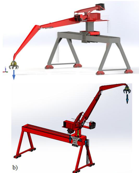
Figure 11. Whole machine with loader crane in two specific geometrical configuration.
