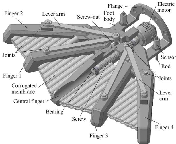
Figure 1. The Foot of Leg of a Walking Robot
