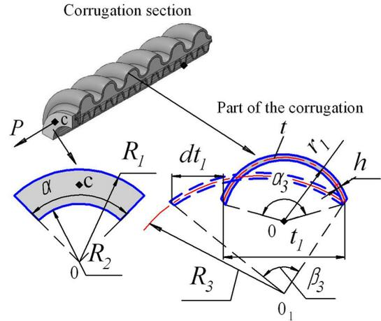
**Figure 5. Cross-section dimensions of corrugated membranes**
