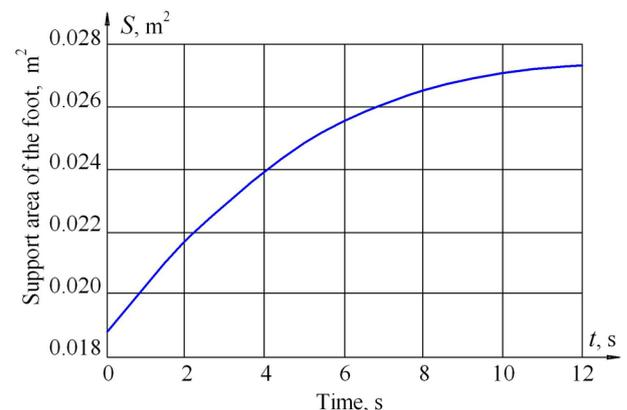
**Figure 8. Graphs of changes in the area of the robot's foot support**
