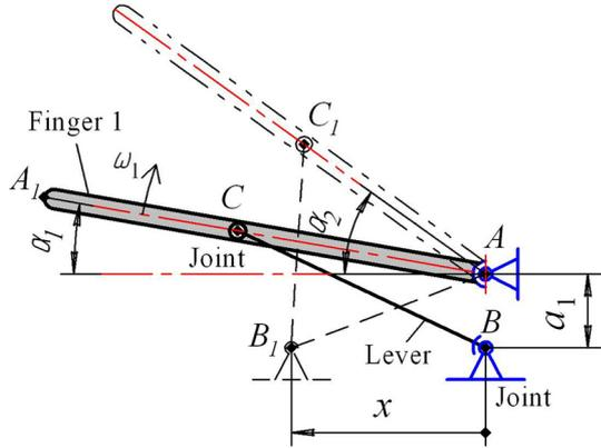
**Figure 3. Kinematic diagram mechanism of the finger 1 with  $AC=\text{Const}$ . (see also Figure 2)**
