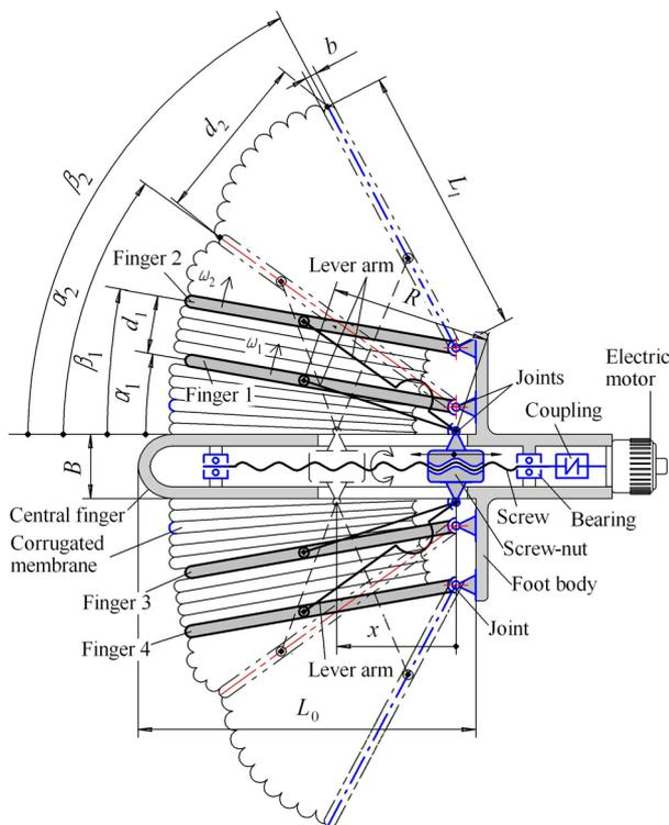
Figure 2. Kinematic diagram of a foot with a variable area of support on the ground
