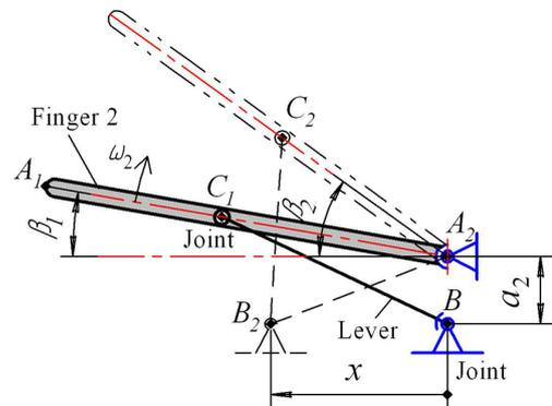
**Figure 4. Kinematic diagram mechanism of the finger 2 with  $A_2C_2=\text{Const}$ . (see also Figure 2)**
