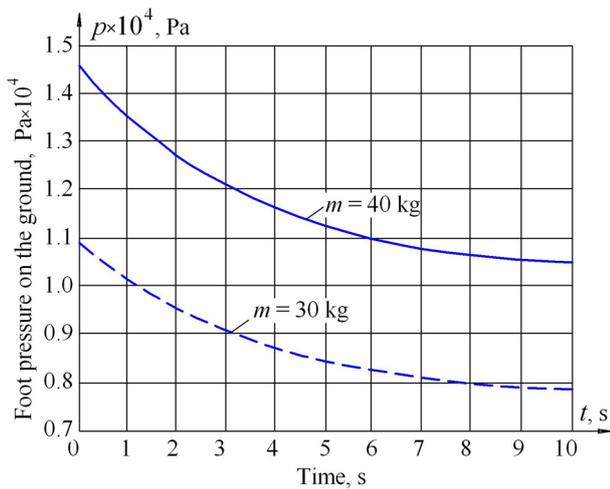
**Figure 9. Graphs of changes in the specific pressure of the robot foot on the ground**
