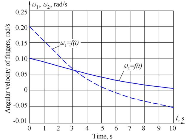
**Figure 7. Change in the angular velocities of the fingers depending on time: at  $a_1=0.02$  m;  $a_2=0.04$  m; lever length  $CB=0.04$  m (see Figure 3); lever length  $C_1B=0.1$  m (see Figure 4)**
