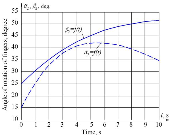
**Figure 6. Graphs of changes in the angles of rotation of the fingers relative to the central finger: at  $a_1=0.02$  m;  $a_2=0.04$  m; lever length  $CB=0.04$  m (see Figure 3); lever length  $C_1B=0.1$  m (see Figure 4)**
