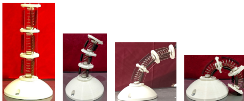
Figure 2. Configurations of the SB-CDCR: (a) initial configuration with zero cable tension; (b) retraction and bending configuration, with all three cables actuated and differential tension applied among them; (c) bending configuration with one or two cables actuated simultaneously; (d) suboptimal bending configuration
