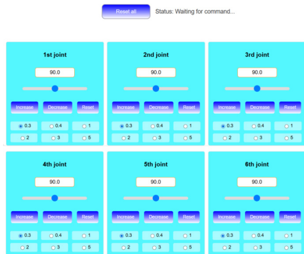
Figure 10. Web-Based Control Interface Using MQTT Protocol for Remote Robot Operation
