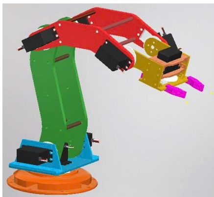
Figure 3. The manipulator design using Autodesk Inventor
