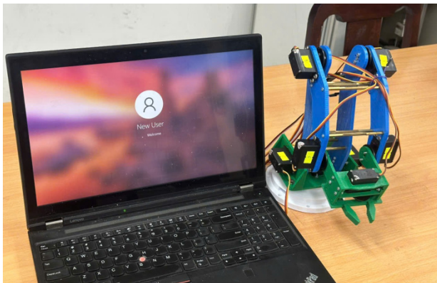
Figure 16. The 3D-printed robotic arm is connected to a laptop running control and vision-based applications.
