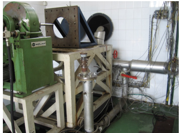
Figure 35. Details of air installation, elements 8, 9 and the brake unit from the Laboratory scheme
