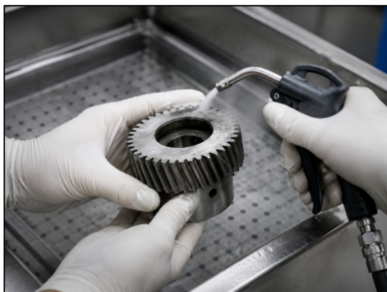
Figure 2. Maintenance Cleaning of Original Helical Gear
