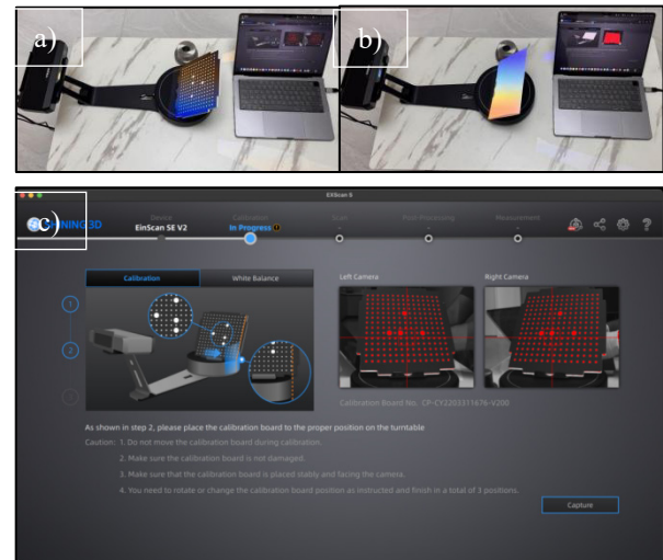
Figure 6. a) Calibration of 3d Scanner. b) White Balance of 3d Scanner. c) EXscan SE V2 Software Interface
