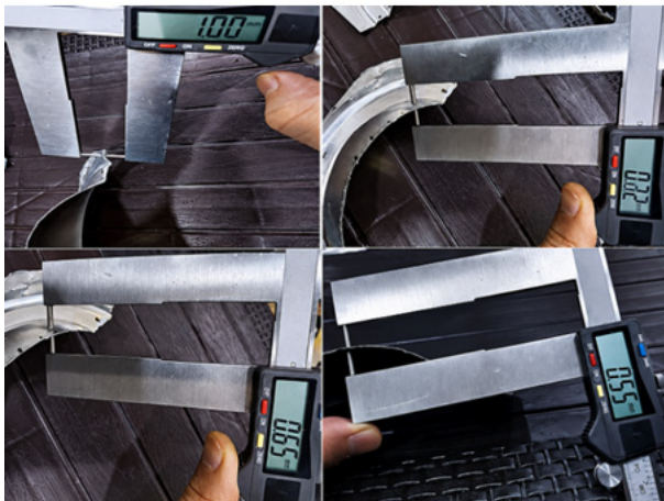
Figure 3. Thickness Measurement Along Selected Points
