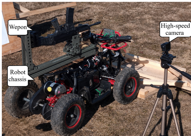
Figure 14. Experimental measurement of robot vibrations.
