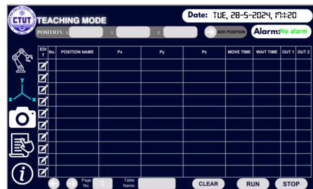
Figure 9. Teaching Mode interface for recording and executing robot positions
