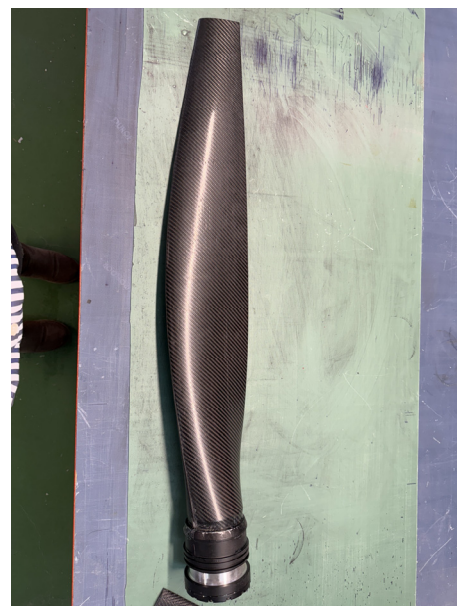
Figure 12. Final composite blade showing the completed laminated structure and smooth aerodynamic surfaces.
