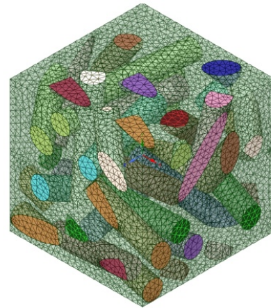
Figure 1. Finite element mesh topology of the stochastically generated 3D random chopped fiber RVE, demonstrating periodic geometric trimming and localized tetrahedral mesh discretization across the fiber-matrix phases.
