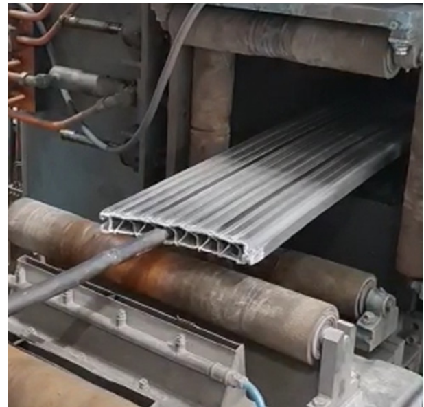
Figure 14. Extruded profile of the final product of carrier panel
